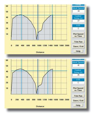
This is run #9. The plot looks very similar to the others we have seen. The Control Delay is 27 seconds, which for this intersection is pretty good. The ending control point is at the far right of the graph, right where the plot is starting to level off. This is the spot most people would place the control point.
