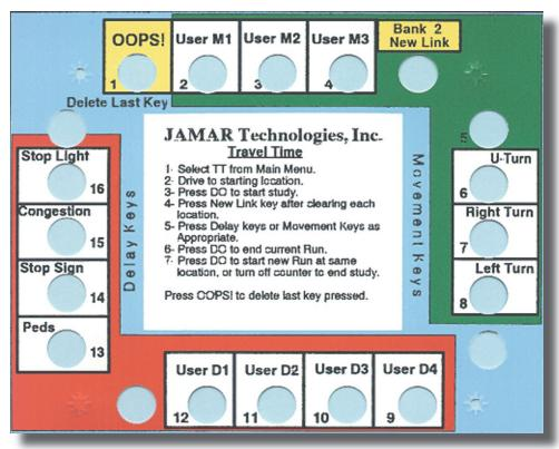
Shown here is the template that you use with the TDC-8 to collect travel time data, which you also use for LOS data. This snaps to the top of the TDC-8 and defines the way the keys on the TDC-8 are used. You only need to use two keys for LOS studies; the DO button to start and stop runs, and the New Link button to mark the stop bar.
