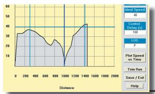
This is run #12. It shows a slower deceleration profile; the control delay clearly starts at around 200 feet while in most of the other runs the delay starts are around 400 feet. Still it is very easy to pick the point where the vehicle first felt the *friction* of the congestion at the intersection.
