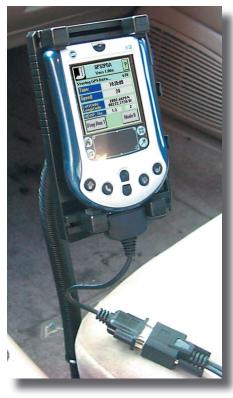
You also can use just about any PDA to collect the LOS data, just about any Palm or Pocket-PC type PDA will work fine. Again, there often are tricks required to figure out how to connect the GPS receiver to the PDA (usually this requires a special cable between the GPS receiver and the PDA), but normally this isn't a major problem.
