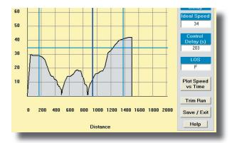
This is run #7. It has a slightly different look. You can see that the vehicle stopped once well short of the stop bar, moved ahead and then stopped again, before finally clearing the intersection. From the Control Delay value (203 seconds) you can see that this vehicle had to wait through two cycles (and this was at 10:47 in the morning!). It is pretty obvious where the delay started and ended for this run so marking the control points is easy.
