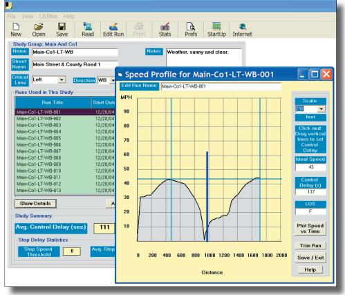
This is the *Run Details* screen for the first run in the study. The graph is a plot of the speed of the vehicle vs distance traveled. You can see that the vehicle was traveling at 30 MPH when the run started. The vehicle increased speed to about 40 MPH and then clearly ran into some congestion. The speed dropped to essentially zero and then increased up to about 42 MPH where it leveled out. This is a typical plot for a vehicle that ran into a red light at a signalized intersection.
