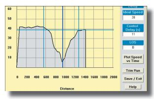
This is a run from a different study. It is included here to show what a run with no stop delay looks like. You treat this run just like the others. In this run the vehicle was cruising along, ran into some congestion approaching the intersection and had to slow down to about 10 MPH at the stop bar, but then accelerated up to the free flow speed. It never stopped so there was no stop delay. This is a good example of why the definition of LOS was changed to
