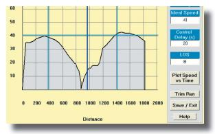
This is run #2. It has almost the same shape as the first run, but the Control Delay is only 20 seconds compared to 137 seconds. This is because in this run the vehicle wasn't stopped for very long at the light, but it isn't obvious from this plot. If a vehicle stops for 3 seconds or 130 seconds the distance plot will still look the same.
