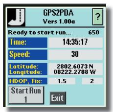
data from the GPS receiver and displays the time, speed, latitude, and longitude on the screen as shown on the screen shot here. It is easy to tell if the hardware is working.
