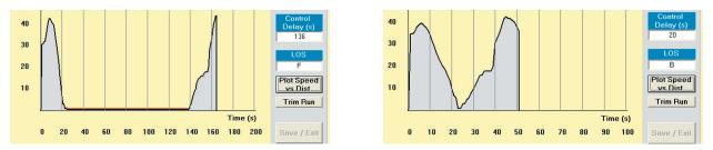
Shown here are the same 2 runs as before, but in Speed vs Time mode. Run 1 is on the left and Run2 is on the right. You can see the long time spent stopped at the light in the first run compared to the much shorter time in the second.
