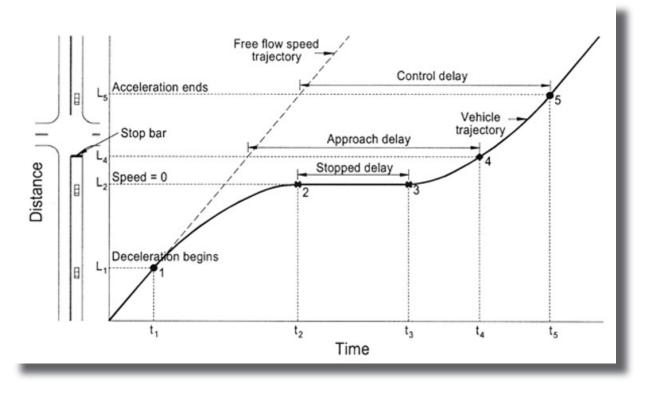
Above is a diagram that shows visually the components that make up control delay. This is a graph of time versus distance traveled as it approaches, goes through, and leaves an intersection. You can see the diagram of the road to the left of the graph.
