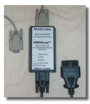
Shown here is a photo of a scantool manufactured by Harrison R & D. It has a cable to plug into the OBD connector in your vehicle and another cable that plugs into the serial port of your laptop or PDA. It sells for less than \$150 and comes with a complete software package to monitor the operation of your vehicle.
