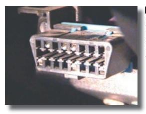
The OBD connector is always the same; it must be located within a few feet of the driver, and it must be accessible without the aid of any tools. Here is a picture of an OBD connector. You probably didn't know it but you have one of these in your car (if it is newer than 1996).
